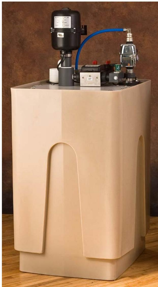
The Bubble-Up XP<sup>®</sup> unit from R.E. Prescott Co., Inc. is designed to remove radon gas from water. Radon is a radioactive gas which can cause serious health problems. Inside the unit, air is injected into the incoming water and allowed to bubble upward. This bubbling action releases the radon from the water. Air containing the radon is then collected, bubbled up and vented out.
