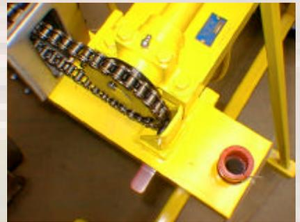
When applying lubrication to the drive gears be careful not to put grease or lubricant on the faces of the drive clutch. Grease gears on the outside of winch housing very lightly. Timely lubrication along with proper chain tension will keep your puller operating for many years.
