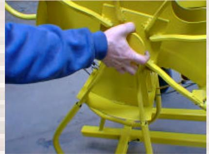
The clutch engages power to the drum. The only force necessary is the spring tension on the lever. Additional force will only damage the clutch mechanism. Turn the clutch clockwise to free wheel the drum. Turn the clutch counter clockwise to engage. Push the power button to operate the drum.
