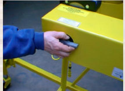
Before freewheeling the drum, disengage the anti-reverse ratchet. With the ratchet disengaged the drum will freewheel in either direction. With the ratchet engaged the drum will only operate in the power up direction. Always operate with the ratchet engaged when pulling pumps.
